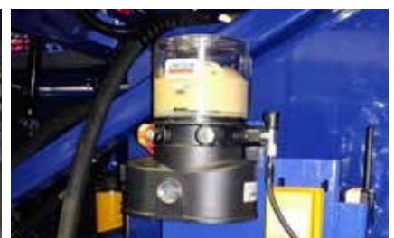
Central Auto-lube System
